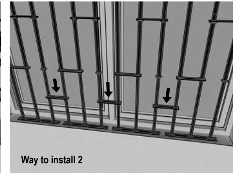
Installing the reinforcement to join one module to the next.
